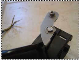
Attach E-clip retainer to pivot pin
